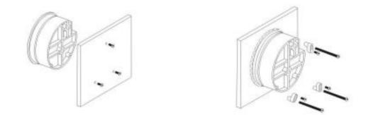
4. For inset installation, drill a good size opening in the mounting plate. Poke the differential pressure gauge in and secure it with the appropriate length of mechanical screw and connector. If the differential pressure gauge is to be mounted on a pipe, please order a pipe mounting kit as an extra.
