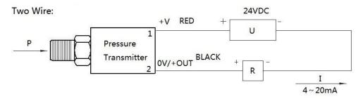
Two-wire 4  $^{\sim}$  20mA current output electrical wiring diagram
