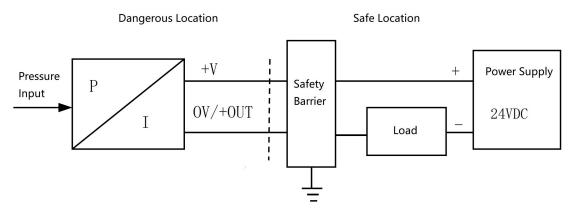
Note: Pressure Transmitter explosion proof spec: Ui=28VDC Ii=93mA Pi=0.65WCi=0.04  $\mu\text{F}$  Li=0
