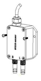
1. This product can be directly installed on the wall or panel using threaded holes.
