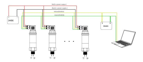
4-wire Modbus-RTU/RS485 (Hirschmann Electrical Connection)
