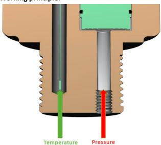
The temperature sensor is a built-in high precision PT100 or PT1000 with a measurement position close to the medium to be measured, a small temperature difference and a fast response. The temperature measurement is also supported by a probe rod structure in order to reach the centre of the temperature to be measured.
